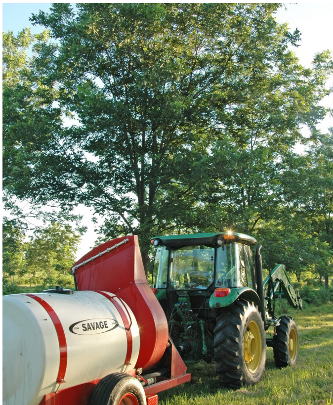
A tractor-mounted air-blast sprayer is designed to reach the upper canopy of mature pecan trees. This type of equipment is essential for achieving full coverage on large trees, but it is rarely practical for most home orchards. Photo by William Reid
